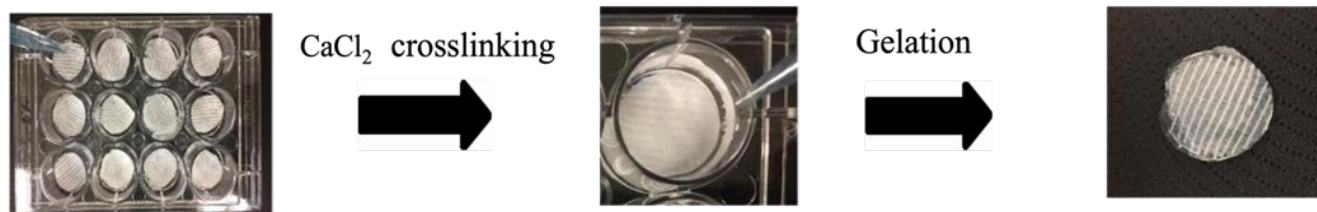
Figure 2 Photograph representation of fabrication of calcium alginate/gauze (CA/gauze)
